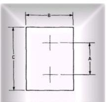
FIG. 13—THE AIMING TARGET for the scope/ laser assembly should be made of dull-finish paper or cardboard. Dimension "A" is the measured distance between the laser beam and the optical center of the scope. Dimensions "B" and "C" are whatever you think will be convenient. The aiming cross-marks should be made with a soft pencil or a medium-point marking pen.
