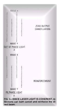
As shown in Fig. 3-a, the beams cancel each other when out of phase (destructive interference). As shown in Fig. 3-b, the beams are additive when in phase (constructive interference). It is the interference between the beams that enables the movement of any reflecting surface to be sensed by a device called a interferometer.
