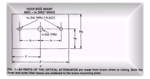
When both filters are in place, rotation of the large-diameter filter-mount will cause a gradual decrease in light transmission (to almost total blockage within 90 degrees of rotation), which allows the receiver to be used over a wide range of light intensities without swamping the photo detector.
